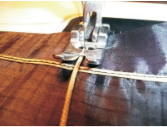
Creating the bridlepoints with reinforcement strings.
